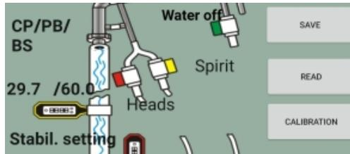
selection valve (Heads) , in this case, on the inscription "Heads", after which you can configure the necessary parameters
