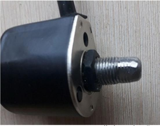
However, it is easier to install the valve “wrong”, that is, with the fitting up, thread down, as in the photo below. The pressure of the alcohol column during selection is not enough to push the valve stem spring, so this is very acceptable in our case.
