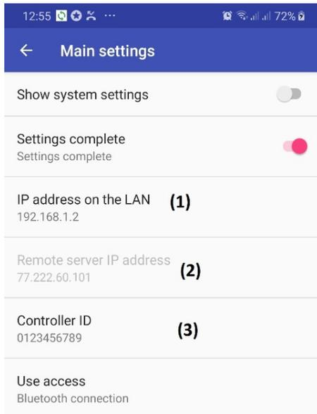
To work in network access you need to set the IP address on the local network **(1)**.
