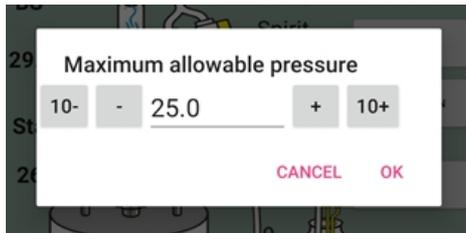
**Note:** To use a pressure sensor, the pressure limit must be set, this is a sign of using the sensor, otherwise its readings will not be read.
