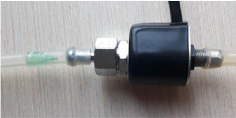
Please note the selection limiter. When using this type of valve, the selection limiter is easiest to use a medical needle that is neatly cut with a file.
