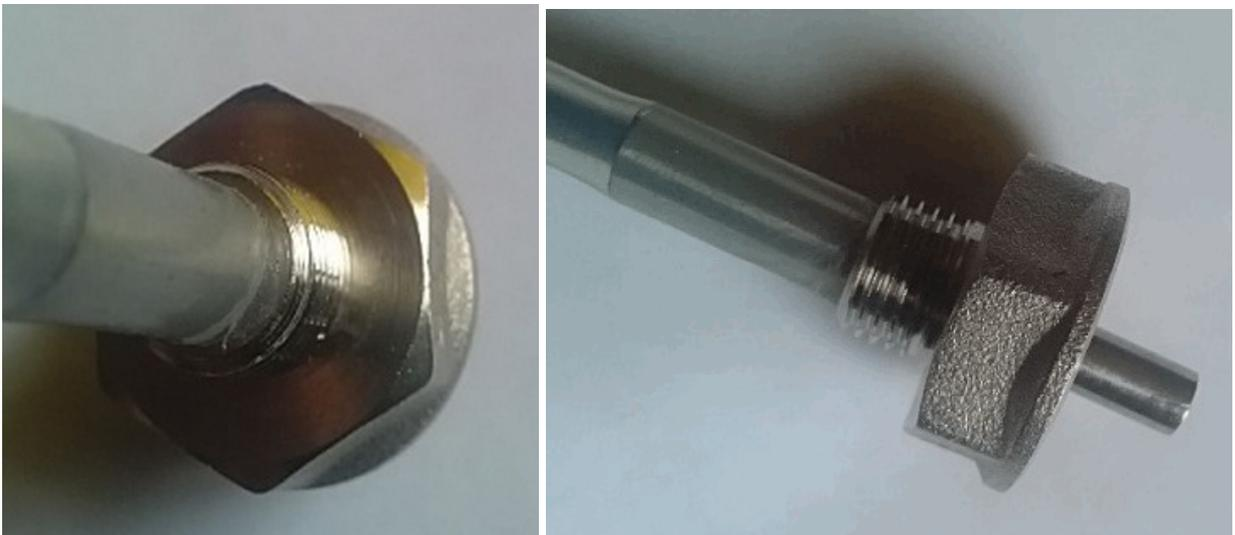
What are the advantages of this method – ease of removal of the sensor, the sensor is protected from the influence of the walls of the sleeve by a silicone tube, that is, the accuracy will be higher than if it touched the walls of the sleeve.
