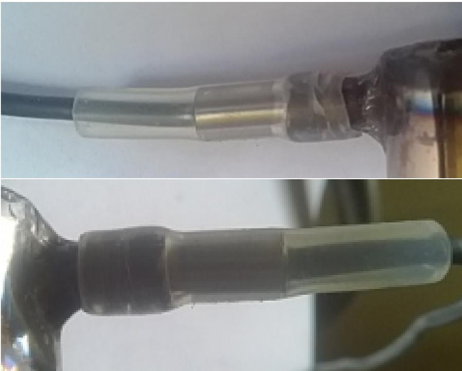
What are the advantages of this method? Ease of installation and removal of the sensor, good tightness of the connection, standard dimensions of the hole for installation.
