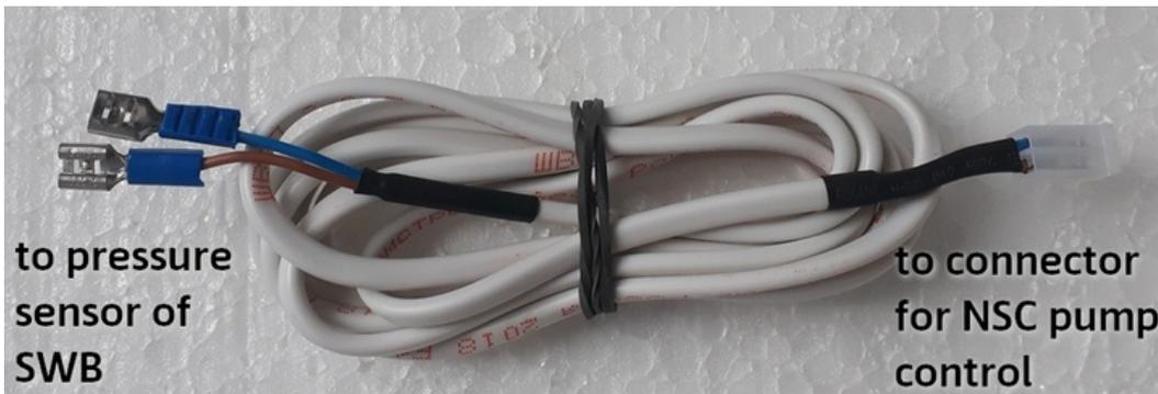
To do this, the connector from the sensor must be connected to the NSC pump control connector, and the contacts to the contacts of the pressure sensor.
