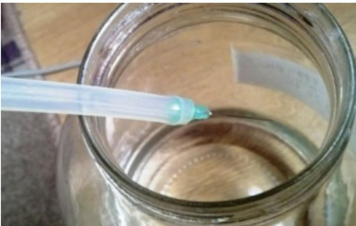
This method has one peculiarity – there should be no air jams in the tube from the valve to the sampling unit, otherwise the selection will be unstable or stop altogether. Air plugs will need to be driven out in some way.
