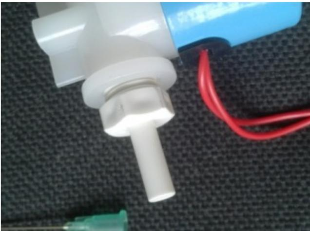
4. Another way to limit selection is with a medical needle mounted on the tube in the receiving container, for example, as in the photo.
