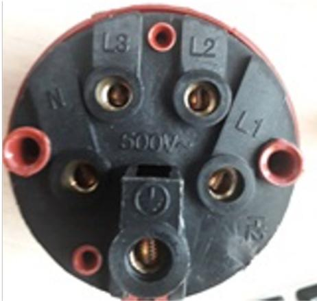
N- Neutral wire, L1, L2, L3 are phases. At the bottom, ground is connected.
